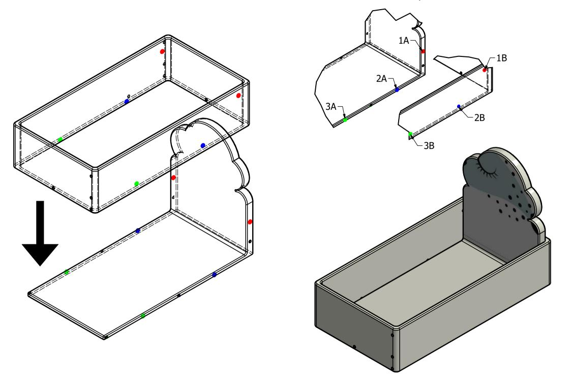
STEP 4: Attach the rattles arch inside the nest and secure with snap buttons
